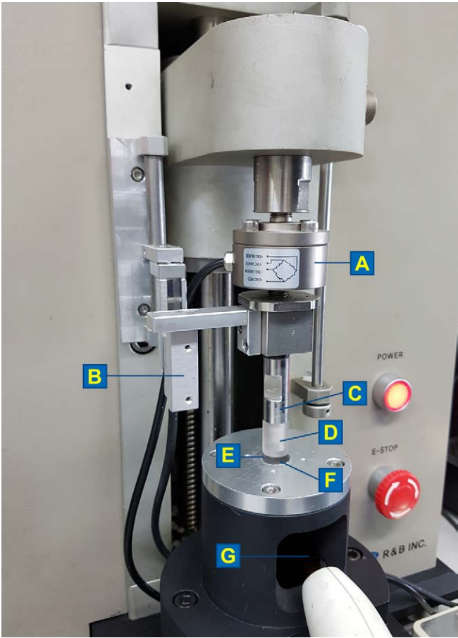
Figure 1. Device for measurement of polymerization shrinkage force and deflection control. (A): load cell; (B): feedback sensor; (C) metal rod; (D) acrylic rod; (E) space for composite specimen placement; (F) acrylic base; (G) light source.
