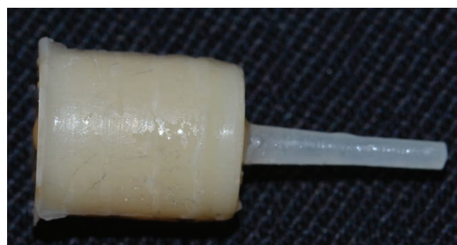
Figure 2. Post bonded to composite resin before being sectioned transversally.
