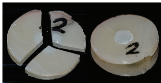
Figure 4. Representation of the predominant failure types after push-out test. (A) Cohesive failure of post and composite resin; (B) mixed failure, adhesive+cohesive of composite resin.
