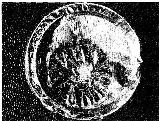
FIG 2. Warpage of tin foil caused by spreading of mercury droplet
