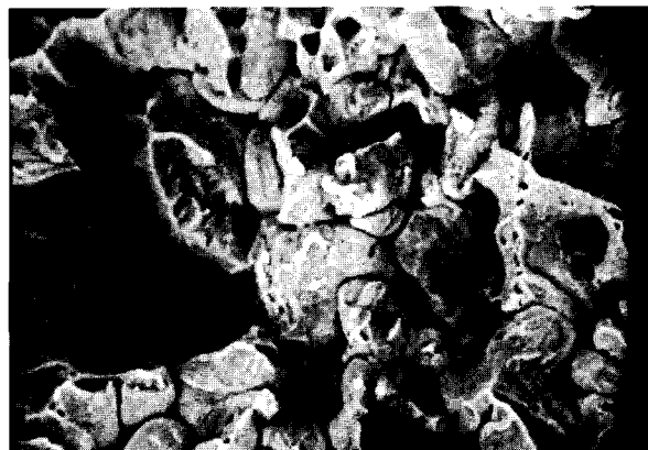
Fig. 7 – Section Showing Transverse Fracture Through Goldent Specimen (2300X).
