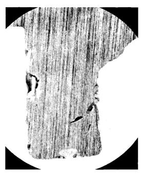
Figure 5. Two 1/64 gold foil pellets compacted with 0.4 mm condenser into convenience pit cut with 0.4 mm end cutting bur. Some porosity is evident in this dense specimen. Longitudinal scratches resulted from metallurgical polishing.
