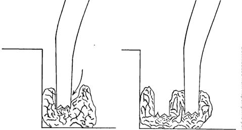
Figure 2. Compaction of a large gold foil pellet with the 0.4 mm monangle condenser. Nib face buried into pellet upon initial impact.
