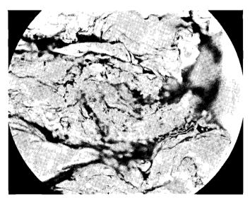
Figure 8. Poorly compacted gold foil at high magnification. Large void spaces are evident between two medium sized pellets. Gold pellets were not spread out prior to impact. The area shown is approximately 0.3 mm in diameter on the specimen.
