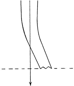
Figure 9. Diagram of  $0.5 \times 0.55$  mm oblique-faced, serrated monangle condenser. Arrow indicates lines of force, parallel with long axis of handle and perpendicular to the nib face.
