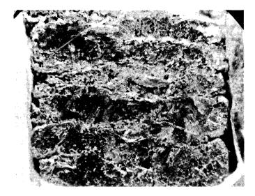
Figure 10. Poorly compacted Goldent specimen. Large pellets were not carefully spread out prior to compaction with the pneumatic condenser and a 0.5 mm servated nib. Layering and a network of porosity are visible. Size of specimen is 2.3 x 2.0 mm.
