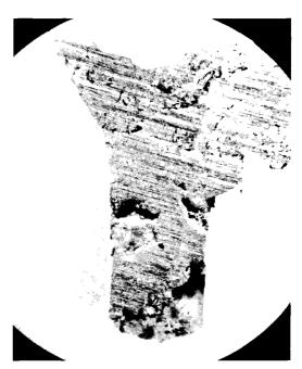
Figure 6. Porous gold resulted from ineffective compaction with the 0.5 mm nib into this convenience pit cut with the 0.4 mm bur. Gold failed to penetrate to the bottom of the pit at the lower right. Large and small voids are evident throughout the mass.
