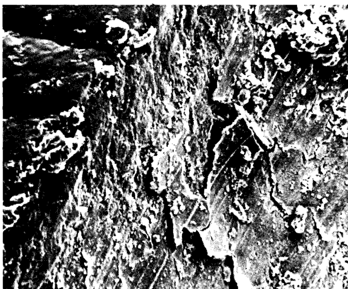
FIGURE 4. Chiselled exit side of cavity prepared with diamond point. Treatment with a sodium hypochlorite solution has resulted in the separation of the apparently smooth surface from the underlying substrate. This could be taken to indicate that this superficial layer has been "smeared" over the underlying enamel but is not firmly united with it. \times 400 . (By courtesy of A. Boyde and the British Dental Journal )
